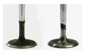
The image shows a gasoline intake valve before and after running on ValvTect Marine Gasoline. The valve on the left is heavily coated in black, carbonaceous deposits and was taken from an engine which had been running continuously on automotive unleaded. In sharp contrast, the one on the right is the same valve after switching to ValvTect Marine Gasoline. Most of the existing deposits have been removed and the previously dirty valve is now virtually as clean as new.
